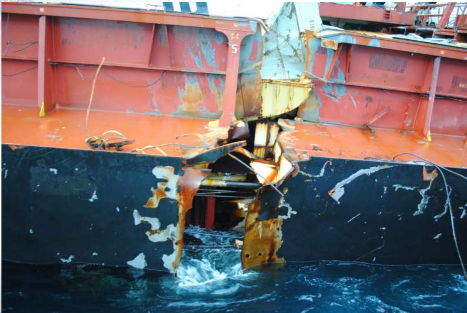
Crack on the starboard side – Frame 191
